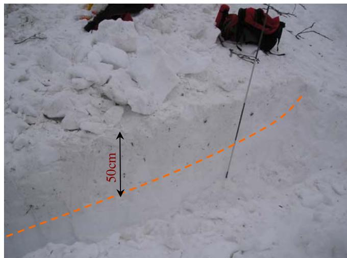
**Fig. 20.** Trench no. 3: The debris concentration decreases gradually towards the front.
