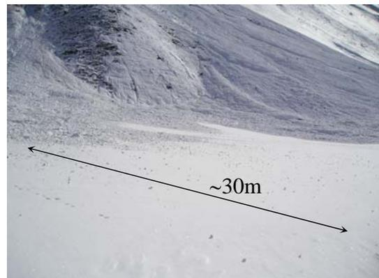
**Fig. 7.** View from trench 1 to the side, showing the flight distances of the soft snowballs.
